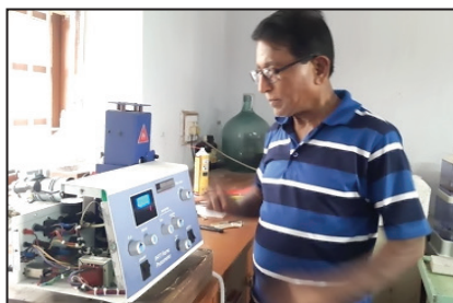
Mr. A.K Chowdhury, NITUB's Instrument Engineer, repairing a flame photometer at BTRI, Srimangal in 2017.
